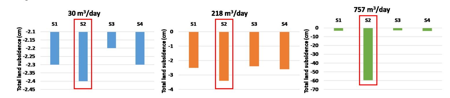
Comparison of total land subsidence caused by pumping at four aquifers by different pumping rates
