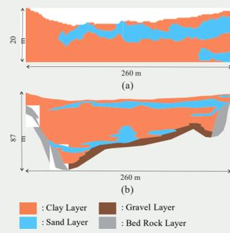
Figure 4. Illustration of complex hydrogeological model of; (a) shallow, and (b) deep soil profile.
