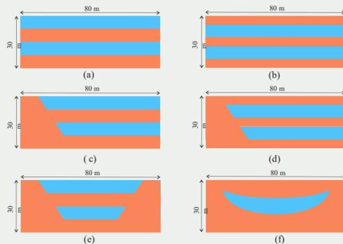
Figure 3. Illustration of synthetic hydrogeological model of; (a) & (b) perfect layer system, (c) & (d) pinch-out (stratigraphic trap) system, and (e) & (f) lens (riverbed deposit) system.
