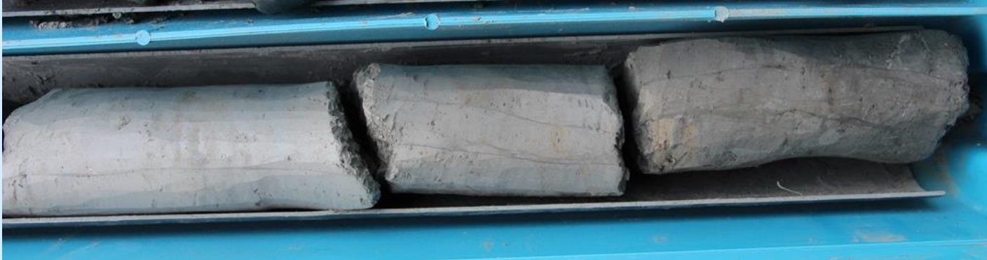
BH-3_31.75~32.00m Layer B, shear plane 85~90°
