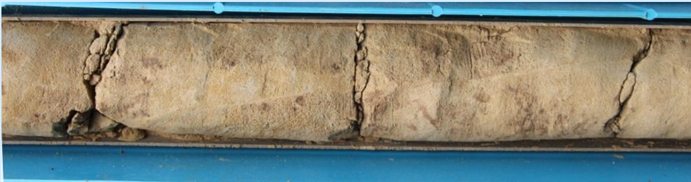
BH-13_3.35~3.65m Layer D shear plane 80°
