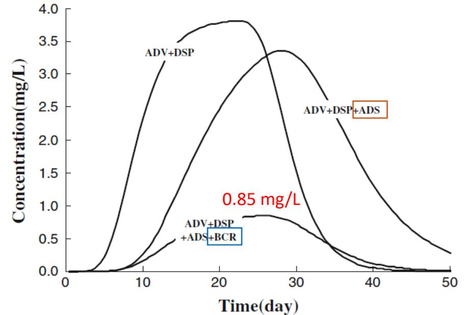
Fig. 8 Breakthrough curves of PCE at observation point
