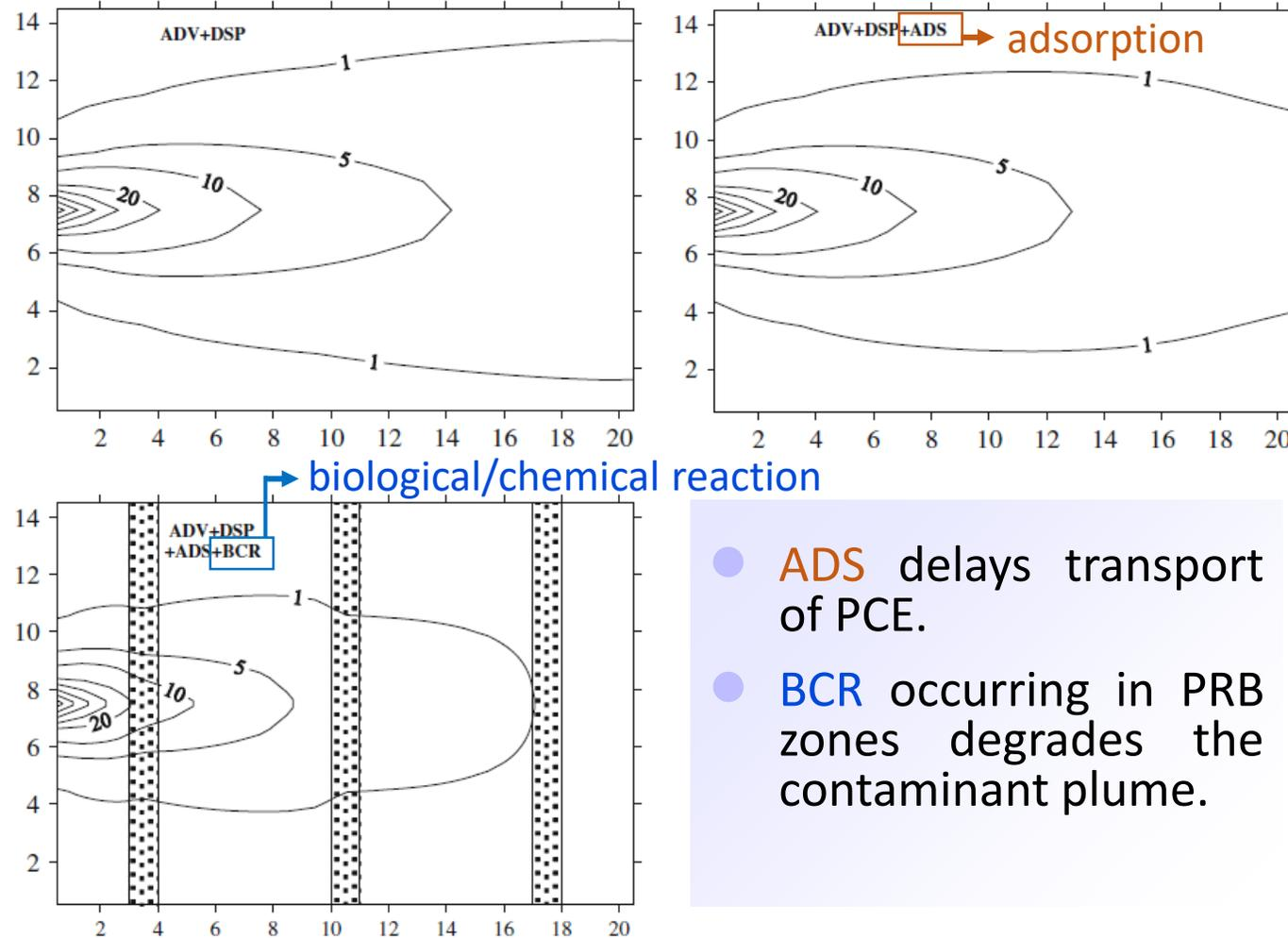
Fig. 7 Concentration profiles of PCE after 20 days at section 1-1 (mg/L)
