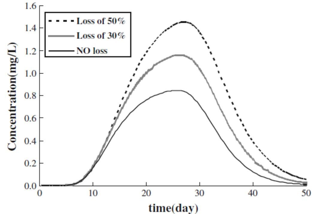
Fig. 18 Breakthrough curves of PCE for sensitivity analyses at observation point
