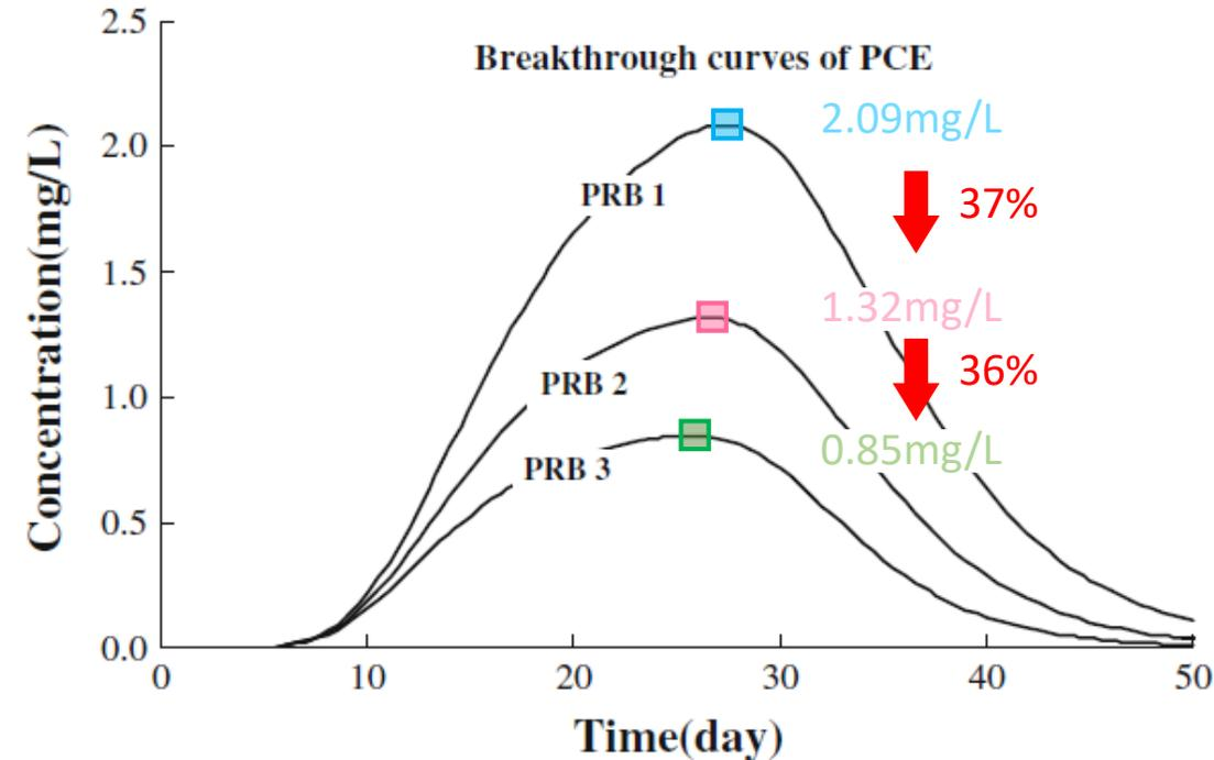
Fig. 10 Breakthrough curves of PCE at observation point
