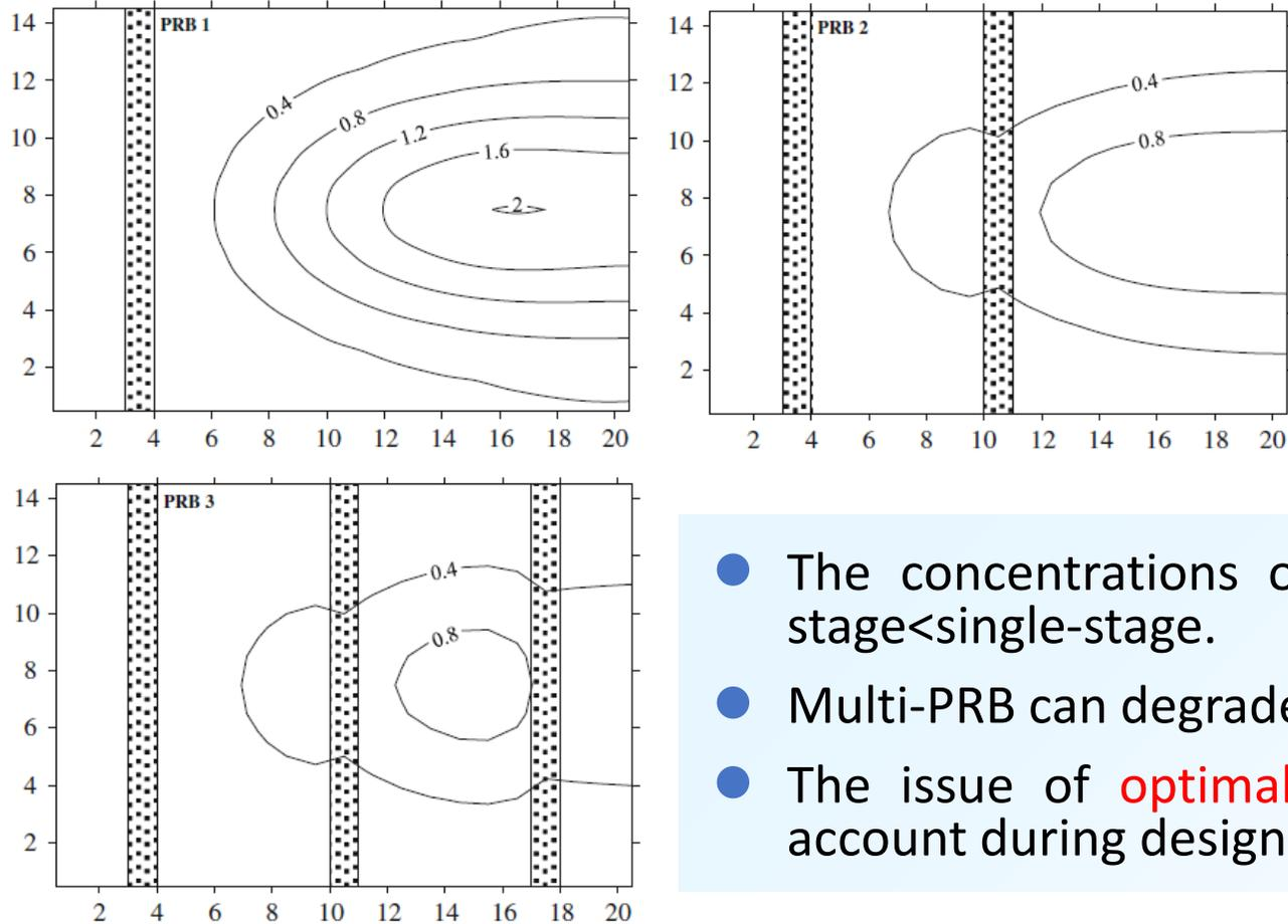
Fig. 9 Concentration profiles of PCE after 30 days at section 1-1 (mg/L)
