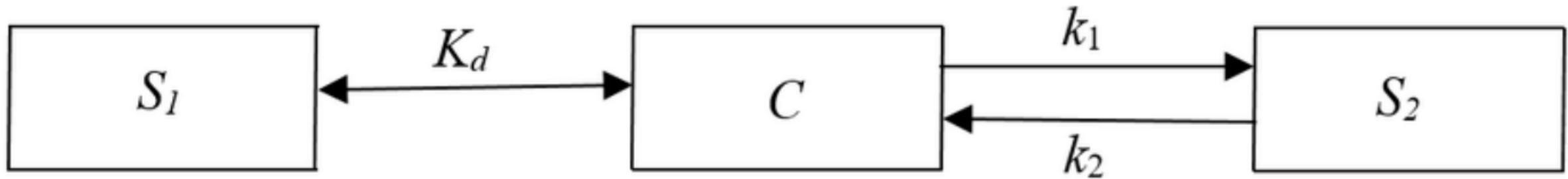
Schematic diagram of the two-site sorption model.  $C$  is the concentration in the solution,  $S_1$  is the amount of solute sorbed on equilibrium sites,  $S_2$  is the amount of solute sorbed on kinetic sites,  $k_1$  and  $k_2$  are the rates of reactions (Zhang and Selim 2005)
