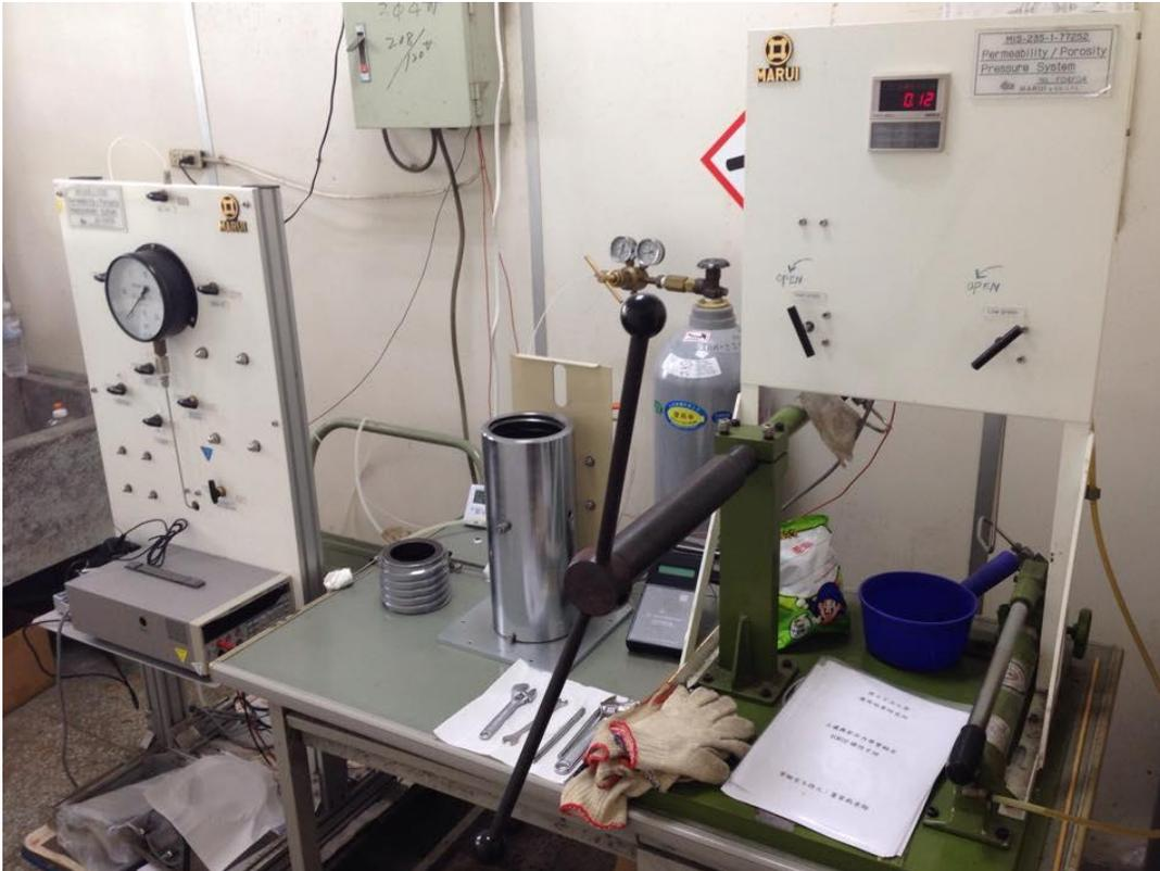
Fig.2 High confining pressure porosity/permeability measuring instrument
