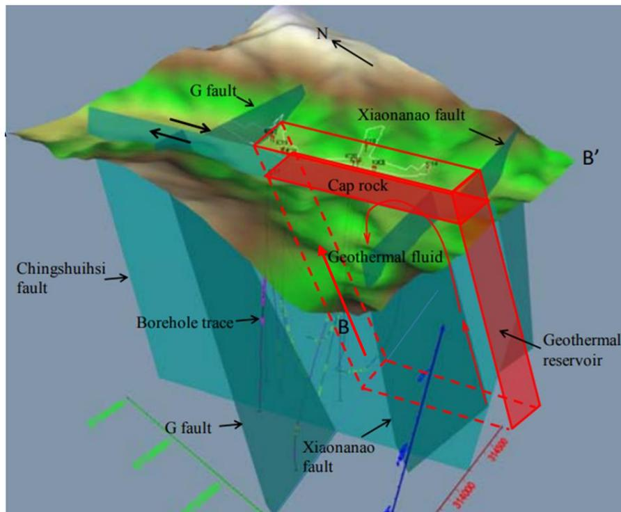
↑ Conceptual model of Chingshui geothermal field (Lee et al., 2012)
