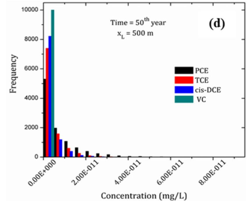
The impact of longitudinal dispersivity on concentration breakthrough curve is analyzed by implementing Monte Carlo type simulations, which could represent the influence of heterogeneity of the porous media on the risk metrics.
