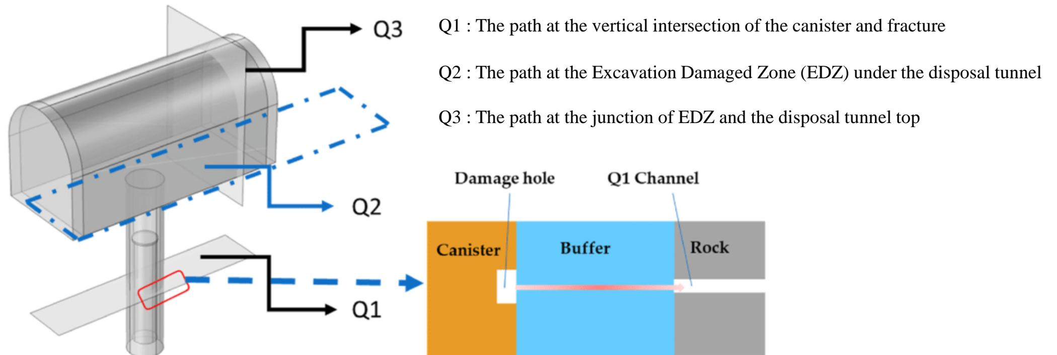
**Fig 3.** Schematic illustration for the Q1-Q3 transport path of radionuclide. (Liang et al., 2021)
