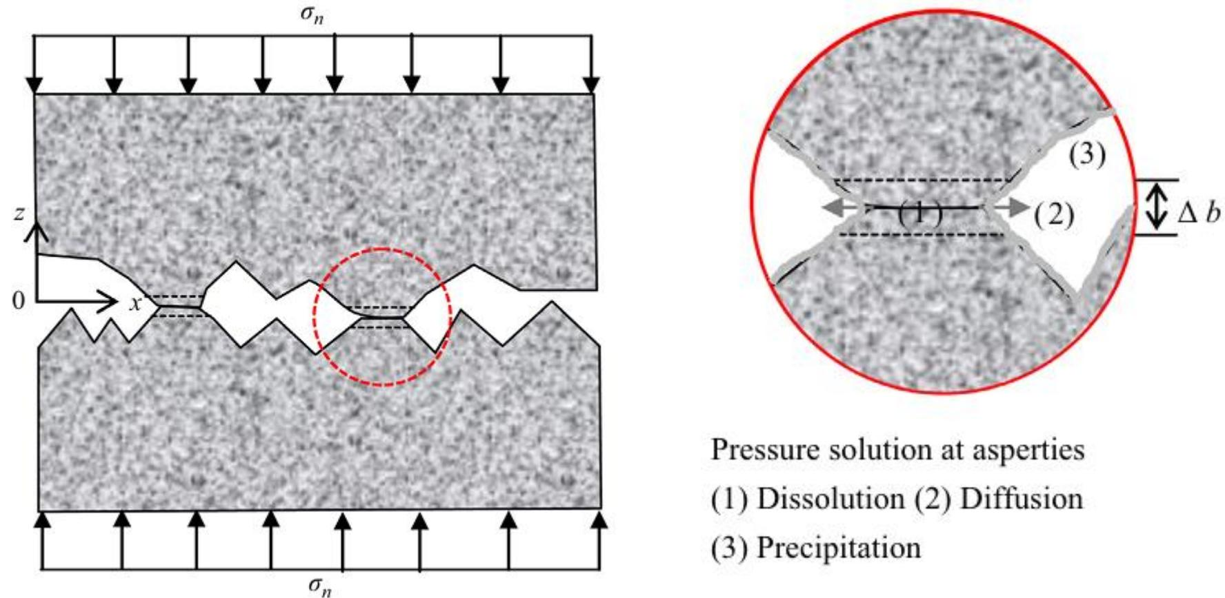
**Fig 5.** Schematic views of fracture aperture reduction due to pressure solution under normal stress.
