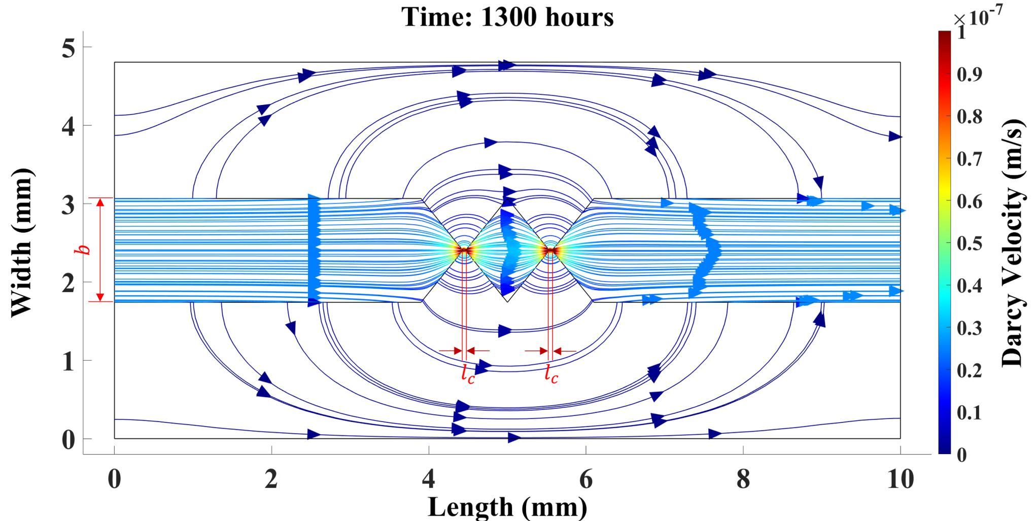
Fracture aperture change after 1300 hours. ( $b = 1.33$ ,  $l_c = 0.03$ )
