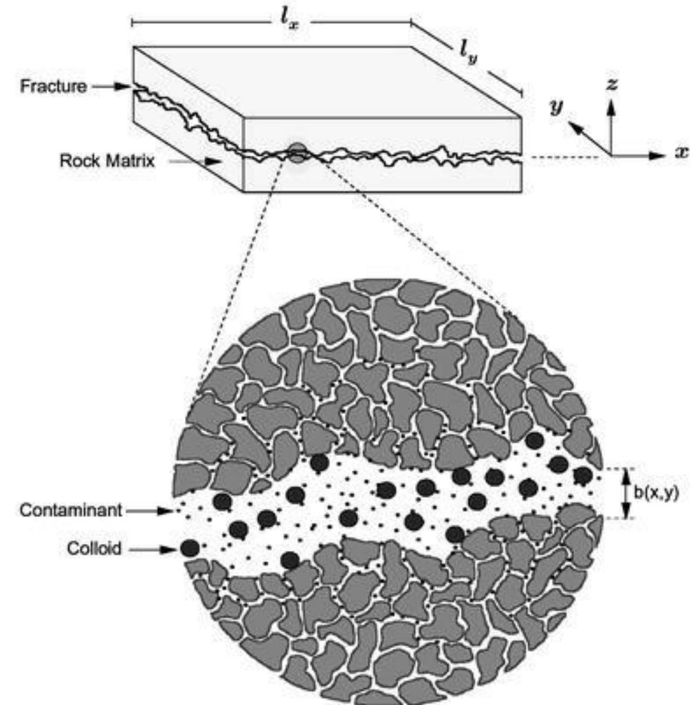
Schematic illustration of contaminant transport in a fracture.
