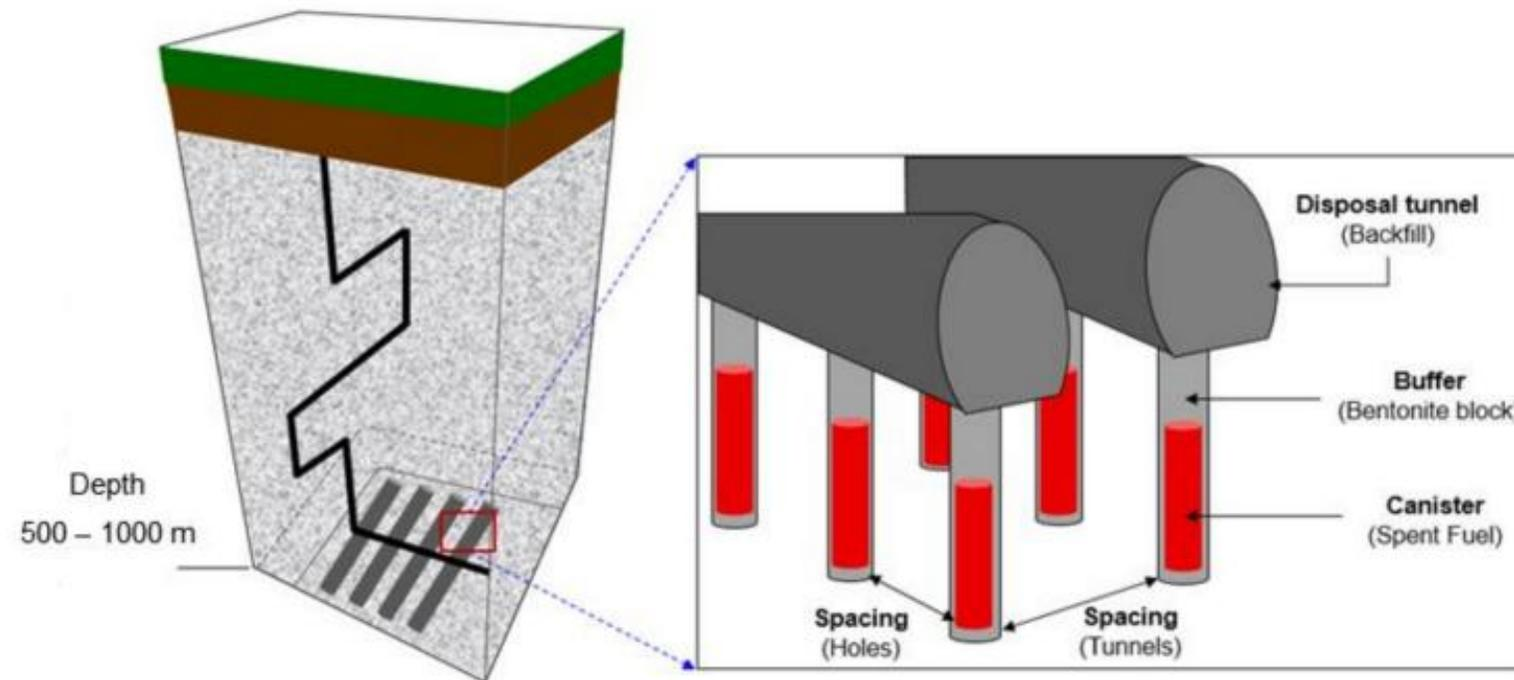
Schematics of deep geological repository and spacing of disposal tunnels and deposition holes. (Kim et al.,2023)
