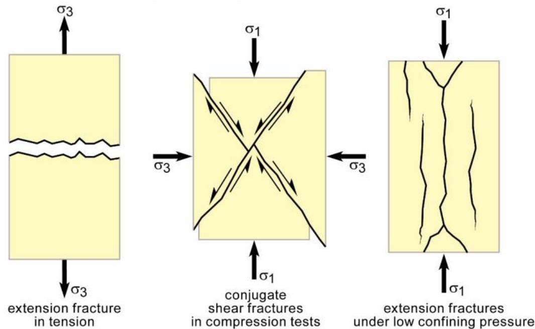
Three types of fractures observed in laboratory experiments (Burg, 2014)
