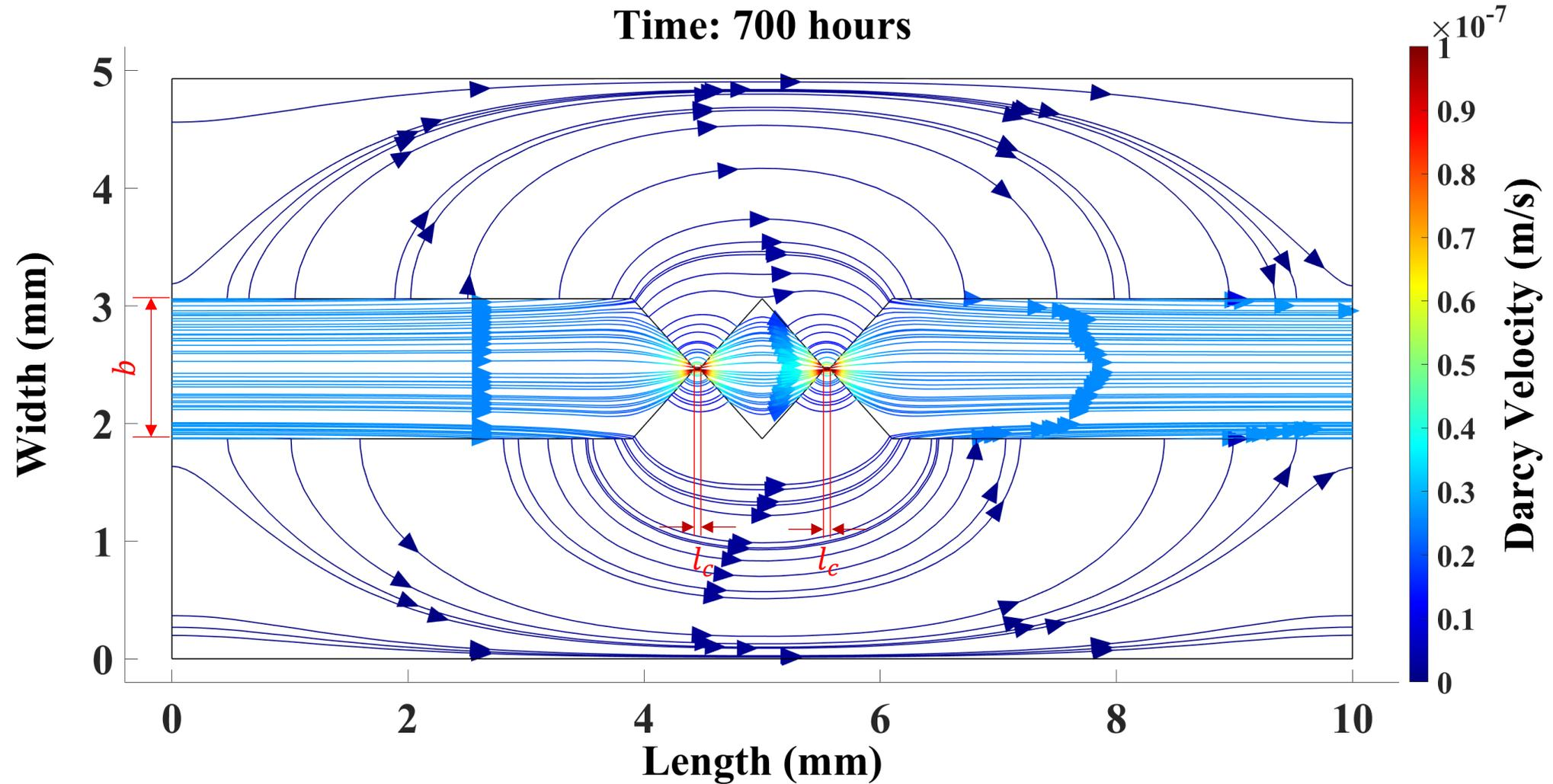
Fracture aperture change after 700 hours. ( $b = 1.19$ ,  $l_c = 0.04$ )
