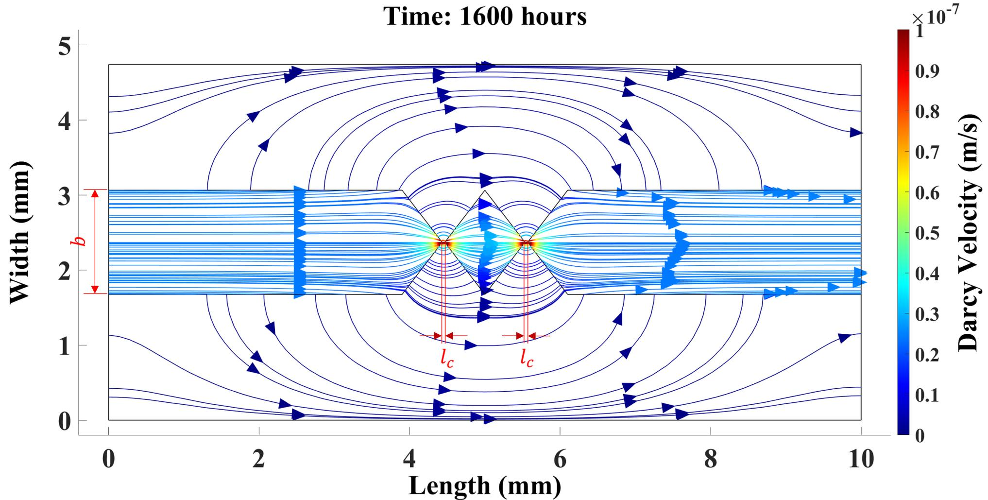
Fracture aperture change after 1600 hours. ( $b = 1.39$ ,  $l_c = 0.03$ )
