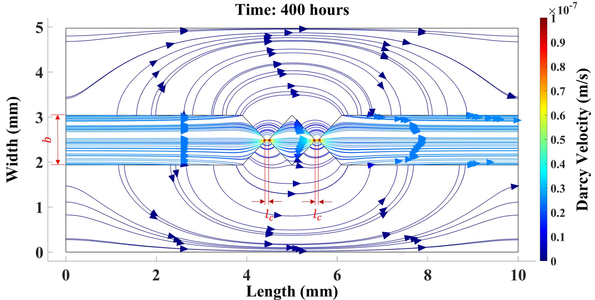
Fracture aperture change after 400 hours. ( $b = 1.11$ ,  $l_c = 0.06$ )
