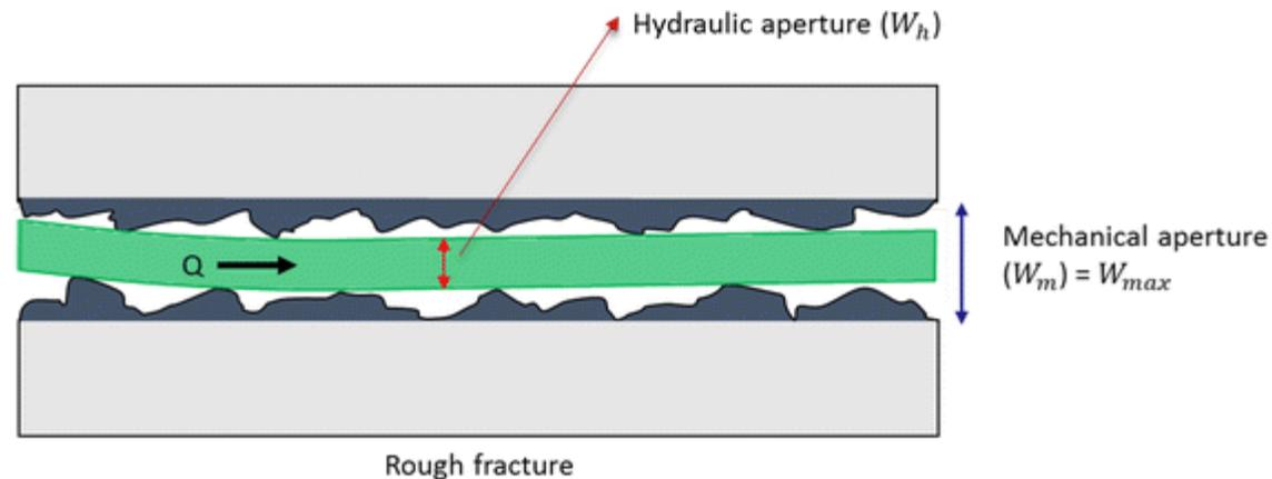
A schematic illustration of fracture hydraulic and mechanical apertures with flow ( $Q$ ) passing through them.
