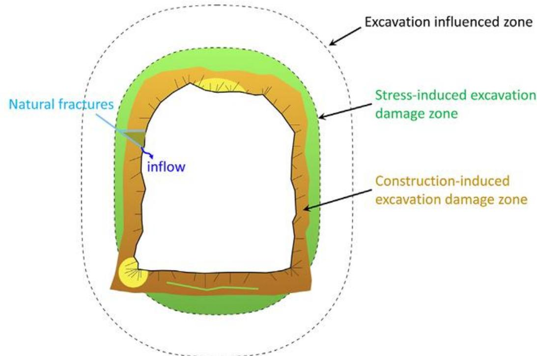
Damage zones in a tunnel constructed using the drill-and blast excavation approach in a generic stress field. (Siren et al., 2015)
