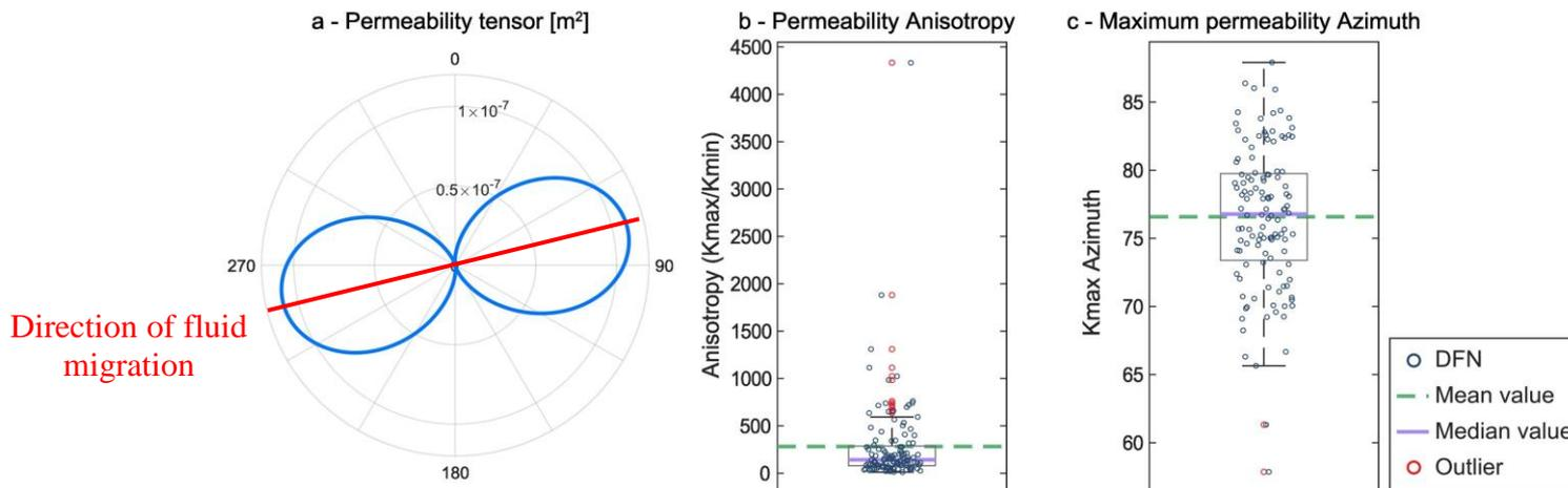
Changes in permeability anisotropy may affect the hydraulic fracturing process.
