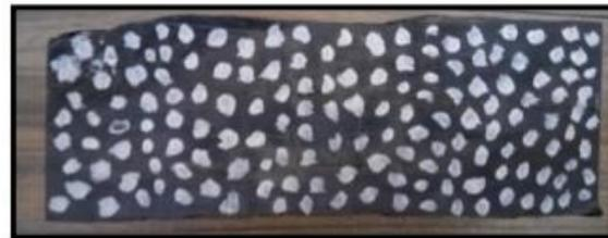
Dot marking on the specimen for PIV analysis
